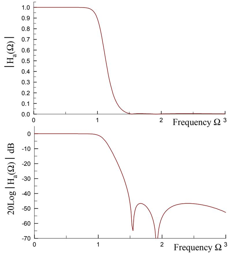
**Figure 4:** Response of a  $N = 7$  order, Type 2 Chebyshev filter with  $\Omega_p = 1$ ,  $\Omega_s = 1.5$ , maximum pass-band attenuation = 1dB (actual is .237dB) and minimum stop-band attenuation = 40 dB. Plots given in normalized amplitude and
