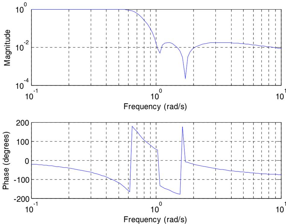
**Fig. 5:** Magnitude and phase response of a 5<sup>th</sup> - order, Type 2 Chebyshev filter with pass-band edge  $\Omega_p = .6$  radian/second, stop-band edge  $\Omega_s = 1$  radians/second, maximum pass-band attenuation = 1dB and minimum stop-band attenuation = 35 dB.
