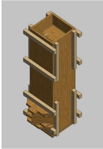
Step 1: Construct and assemble the Wood Mold
