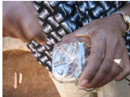
*There are several types of simple hand washer. This one uses a plastic bottle. Cut the bottom off about one third up. Make a hole in one corner of the base.*
