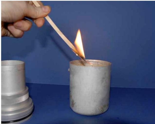
Light the methanol carefully with a taper.
