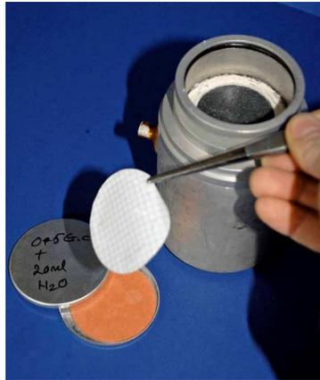
Then quickly open the petri dish and add the membrane, grid side up.
