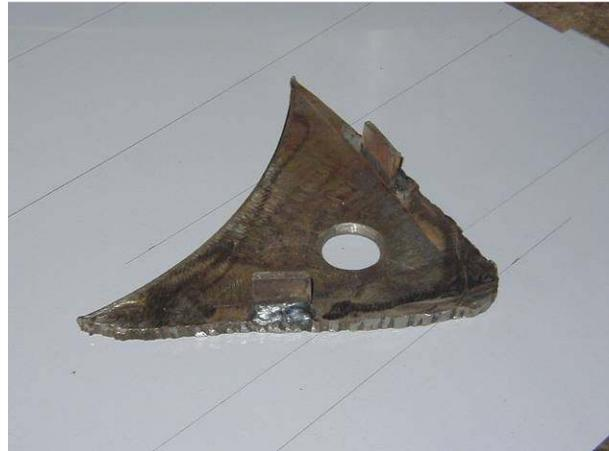
For the nose itself, take the 265mm x 260mm x 2mm plate and draw and cut as per drawings in the Annexes. Fold in centre and grind to shape.
