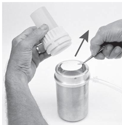
Remove the membrane from the filter head
