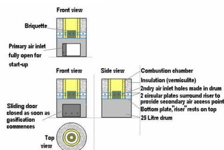
Figure. 33. The Holey Briquette Gasifier Stove.
