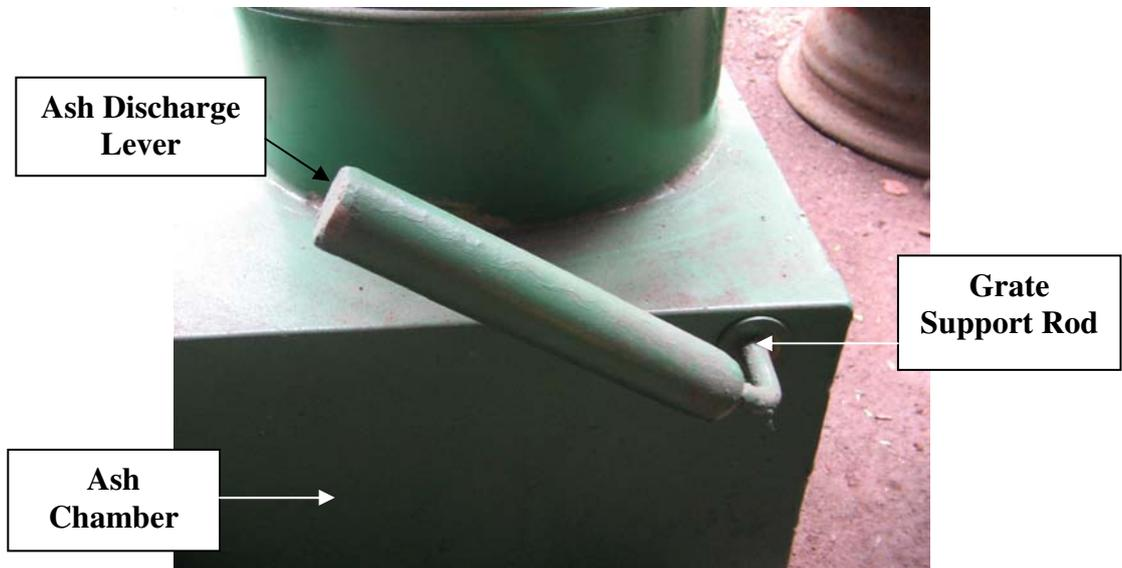
Close Up View of the Ash Discharge Lever
