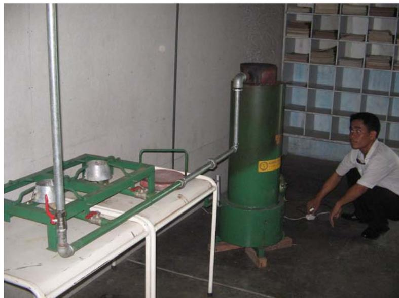
Figure 83. The Table-Top Multiple “Remote Burner” RHGS
