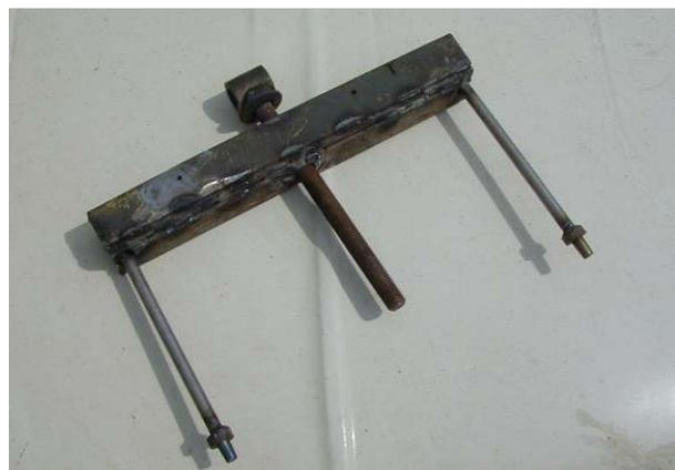
Take two pieces of 40mm diameter x 50mm long BMS rod and drill 18mm holes lengthways through each – these are the puller locking bushes.
