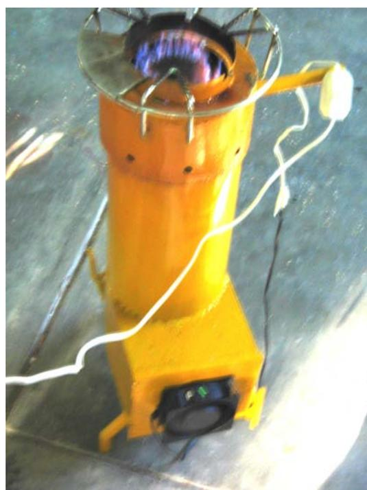
Figure 19. The CPU Proto-Type IDD/T-LUD Rice Husk Stove Model 1.
