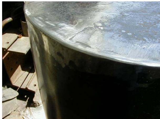
**Step 4 – Bending the top and bottom rings for the outer shell**
