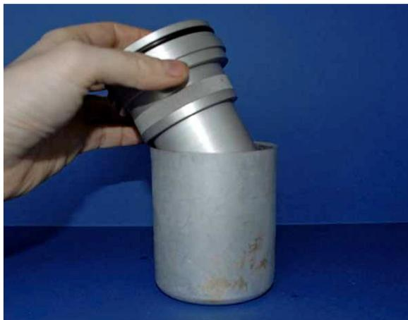
Quickly invert the filter assembly into the cup and leave it for 15 minutes for the vapour to sterilise the apparatus.
