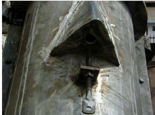
Take the flat for the nose plate lock (25mm x 40mm x 6mm) and drill a 13mm hole in the centre. Weld an M12 nut to the base spanning the hole. Then weld this piece to the outer shell 40mm below the nose plate position. The nose plate will be held in position using a 75mm long M12 threaded bolt.
