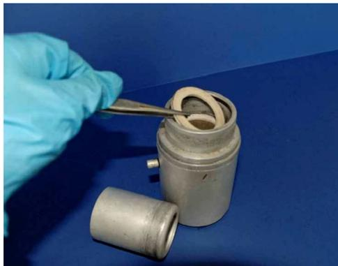
Remove the top part of the filter assembly.
