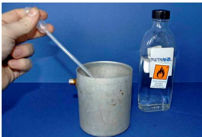
Add ~ 1ml methanol to the cup with a pipette,
