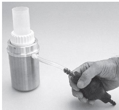
Attach the vacuum pump and create a vacuum to draw the sample through the membrane
