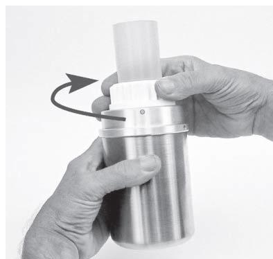
Fit the filter funnel and plastic collar
