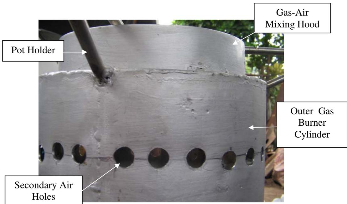
Close Up View of the Secondary Air Inlet Holes
