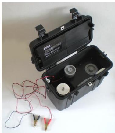
Connecting the kit to an external battery using the crocodile clips connection
