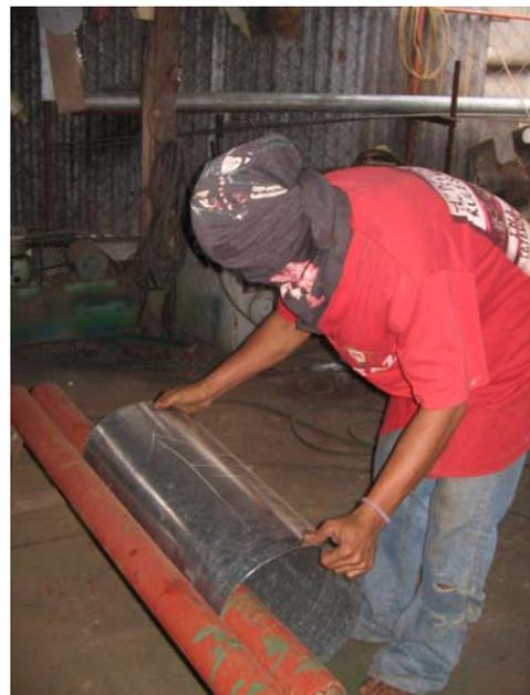
Figure 56. Forming Cylinders on Pipe Bender.
