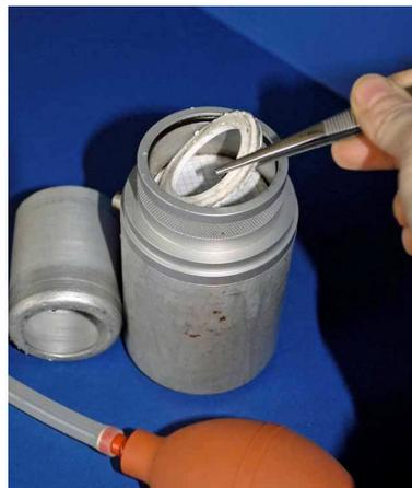
Disassemble the funnel and remove the top ring with tweezers...
