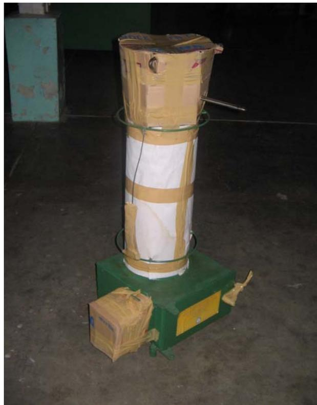
Figure 62. The Stove Wrapped with Thick Paper Ready for Shipment.
