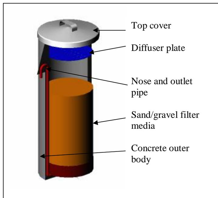
**Figure 2 Cut away view of the Round Bio Sand Filter**
