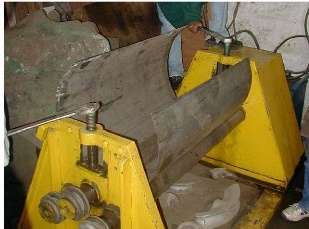
Produce a cylinder of 354mm outer diameter.
