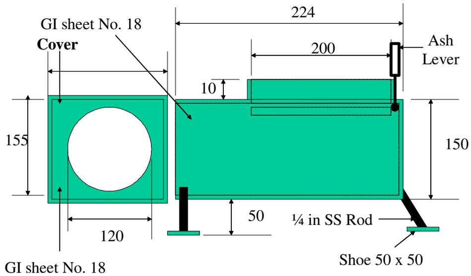
Longitudinal View of the Ash Chamber
