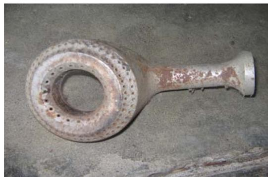
Figure 44. The Conventional LPG Burner.
