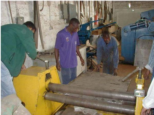
In a three-roll bender roll the plate for the outer shell
