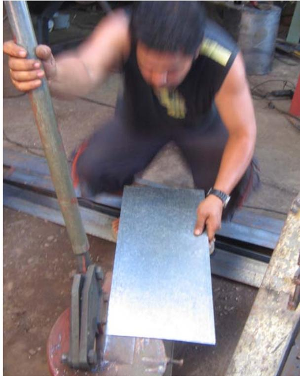
Figure 55. Cutting Metal Sheet with Bench Snip.
