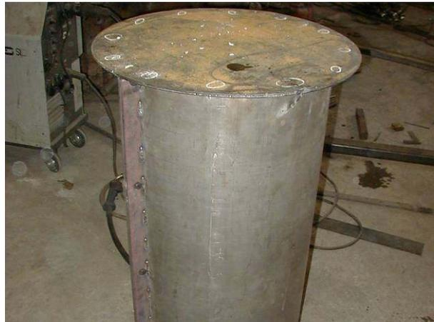
Next, take two of the outer shell locking flats made in the step 5 and tack-weld one on either side (the side of the original joint and opposite).
