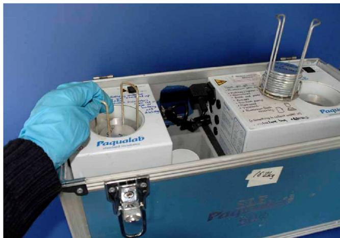
Add the dishes to the incubators, put on the lids and leave for 16 hours.
