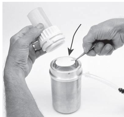
Place the membrane onto the filter support
