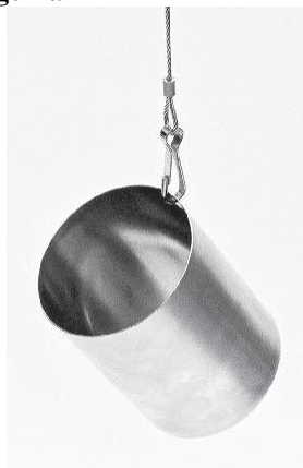
Fasten the sampling cable to the sample cup
