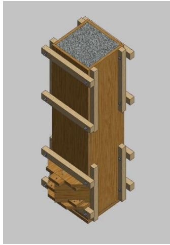
Step 2: Mix and pour concrete into the Mold, let it sit overnight
