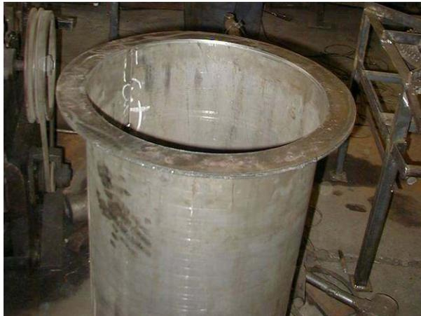
Take the top and bottom rings for the outer shell that were made in step 4 and weld them to the top and bottom of the outer shell cylinder made in step 1.
