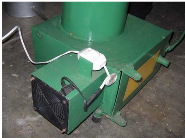
Figure 8. The Fan Assembly.
