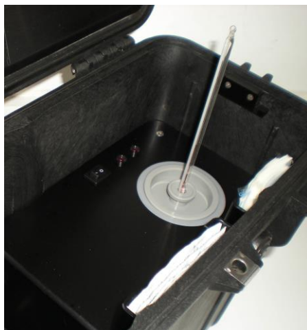
Incubator fitted with testing lid and thermometer assembly
