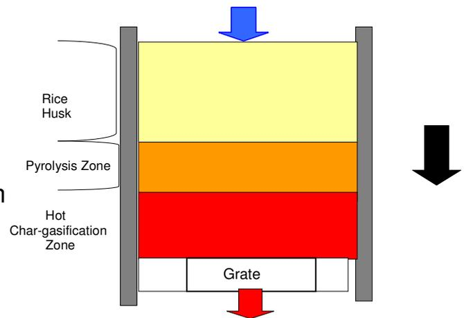
Figure 36 A. DownDraft Type Gasifier. (Bottom-Lit)
