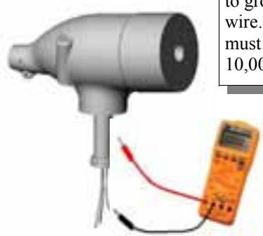
Check resistance to ground on any wire. Resistance must exceed 10,000 ohms.
