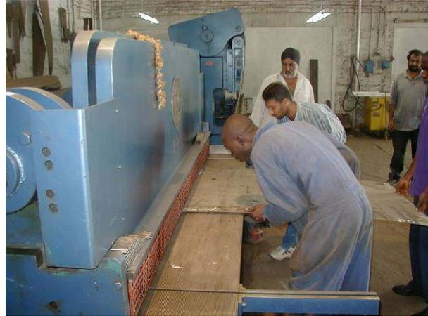
Cut the plate for the outer shell body to the right size.
