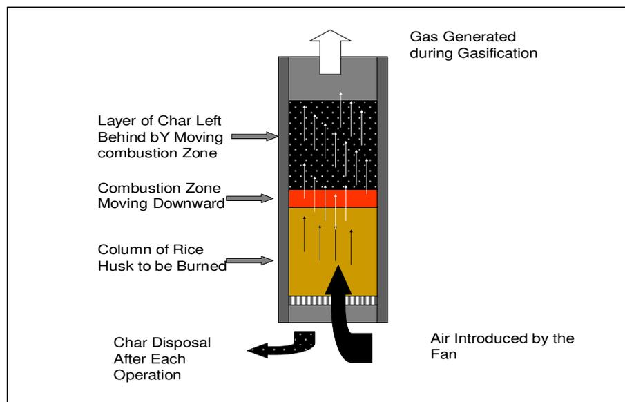
Figure 10. Schematic Drawing of the Principle of Operation of the Rice Husk Gasifier Reactor.
