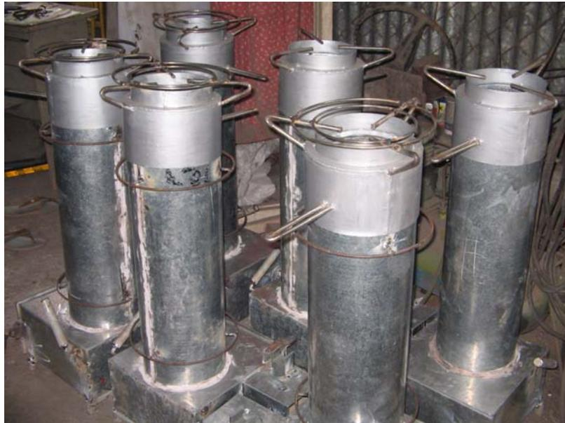
Figure 59. Completely Fabricated Six Units Rice Husk Gas Stoves.
