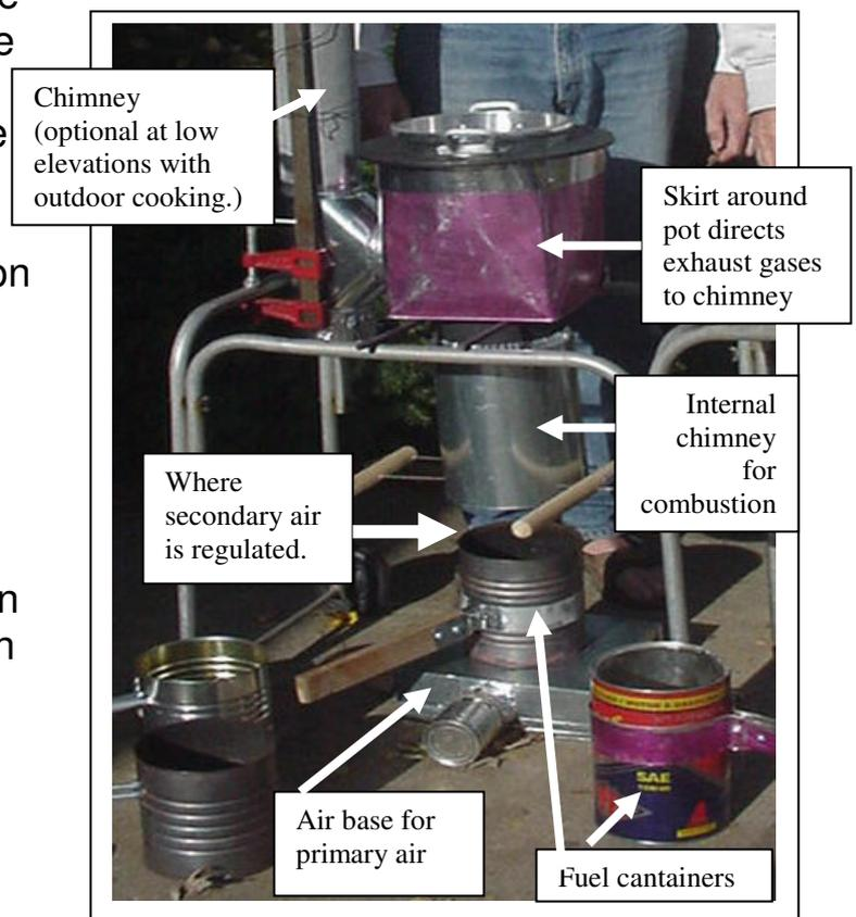
Figure 27. An improved Juntos Model B T-LUD gasifier stove, including chimney needed for altitudes above 1000 meters.
