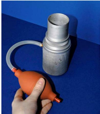
Attach a vacuum bulb (make sure it's the right way round!) and squeeze to draw the water through the filter.
