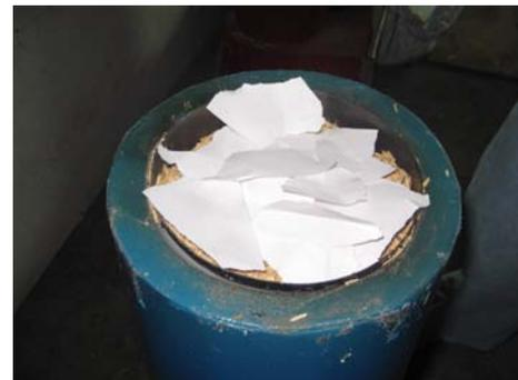
Figure 72. Placing Small Pieces of Paper on the Fuel Column.
