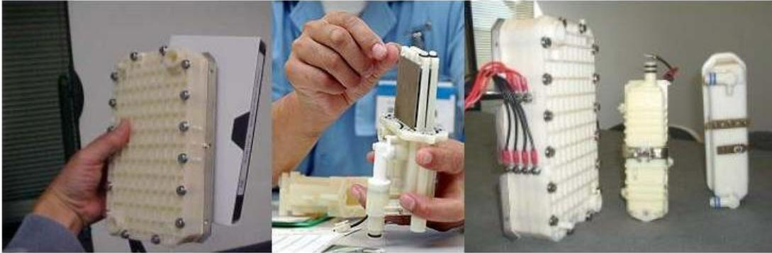
A detailed look at the 3-layer filter & 7 electrode plate electrolysis chamber of the SD501
