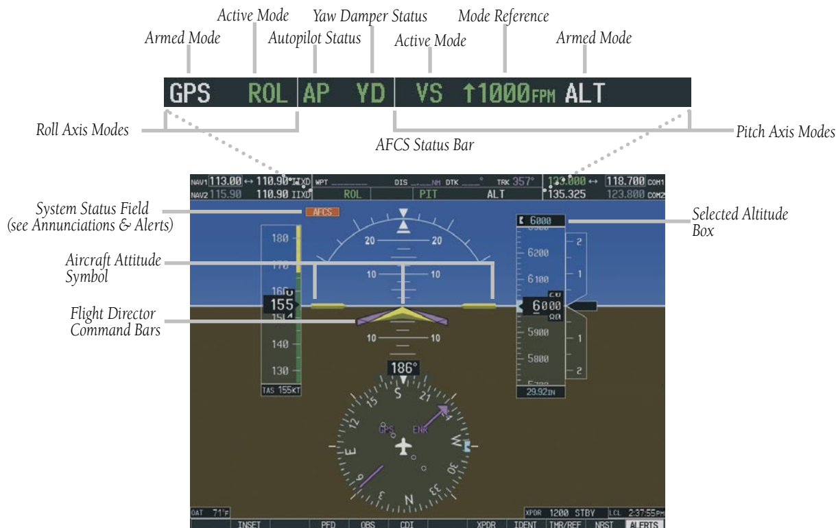
Figure 6-3 PFD AFCS Display
