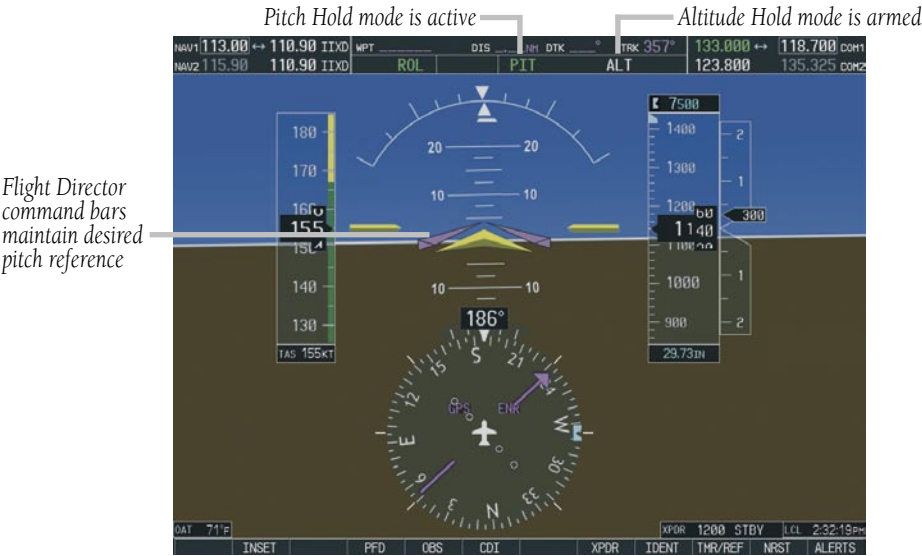
Figure 6-12 Pitch Hold Mode
