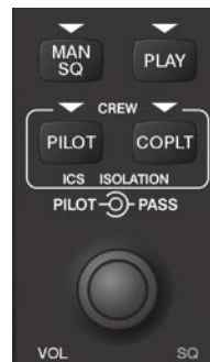
Figure 5-7 Volume/Squelch Control
