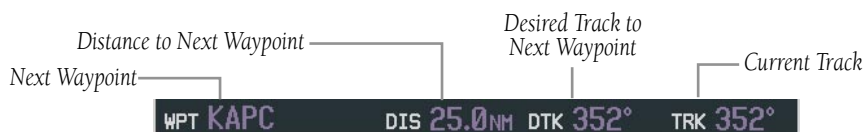
Figure 2-3 PFD Navigation Status Window
