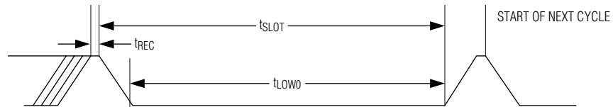
1-Wire WRITE-ZERO TIME SLOT
