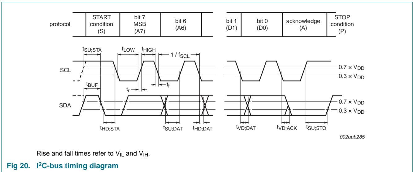
Fig 20. I<sup>2</sup>C-bus timing diagram
