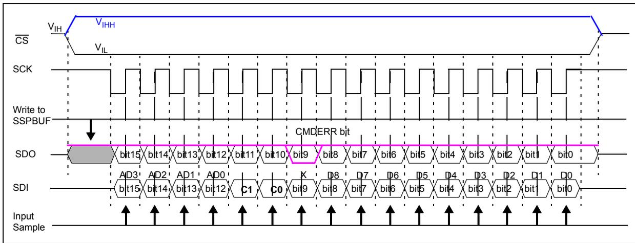
FIGURE 6-3: 16-Bit Commands (Write, Read) - SPI Waveform (Mode 1,1).
