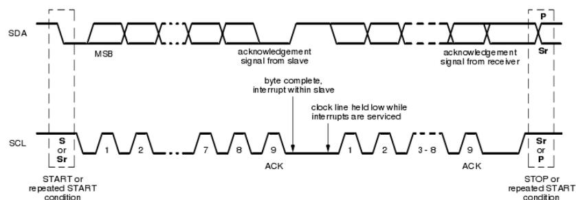
Figure 7: I<sup>2</sup>C Bus data transfer
