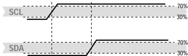
**Figure 12** Transmission Stop Condition (P) - a low to high transition on the SDA line while SCL is high. The Stop condition is a unique state on the bus created by the master, indicating to the slaves the end of a transmission sequence (bus is considered free after a Stop).
