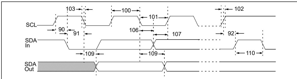
**FIGURE 1-4:** I<sup>2</sup>C Bus Data Timing.
