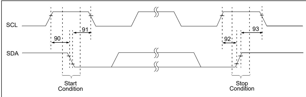
**FIGURE 1-3:** I<sup>2</sup>C Bus Start/Stop Bits Timing.
