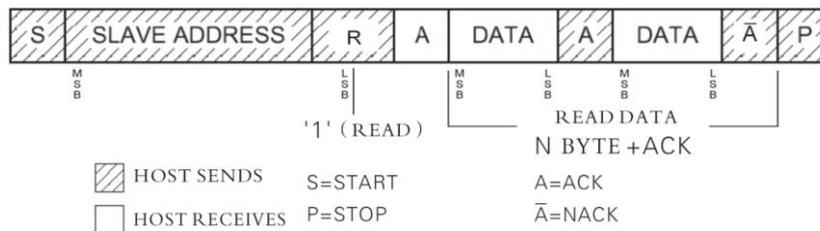
Figure 11: I<sup>2</sup>C The bus master receives data from the slave's basic format
