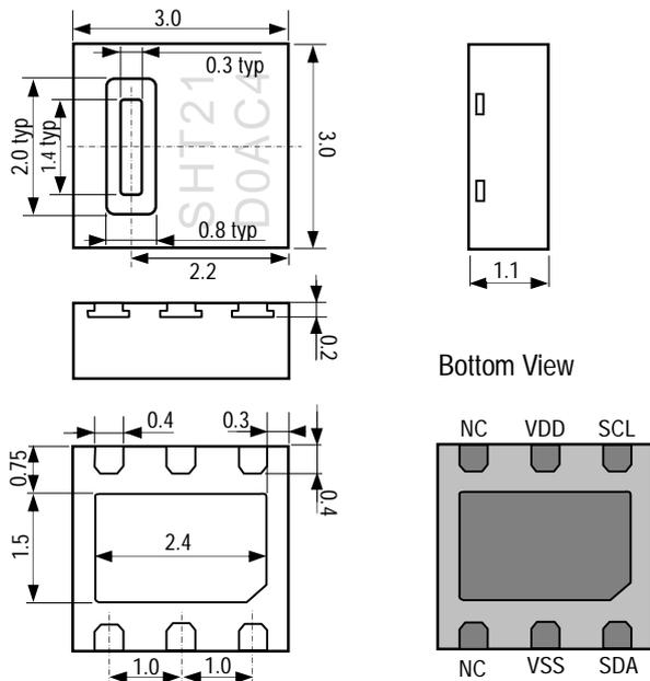
**Figure 1:** Drawing of SHT21 sensor package, dimensions are given in mm (1mm = 0.039inch), tolerances are  $\pm 0.1$ mm. Die pad (centre pad) is internally connected to VSS. NC are floating. VSS = GND, SDA = DATA.
