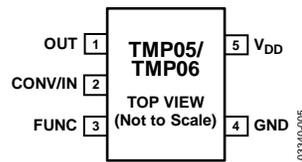
Figure 5. Pin Configuration
