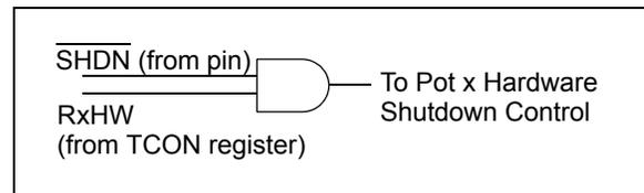
**FIGURE 5-3:** RxHW bit and  $\overline{\text{SHDN}}$  pin Interaction.
