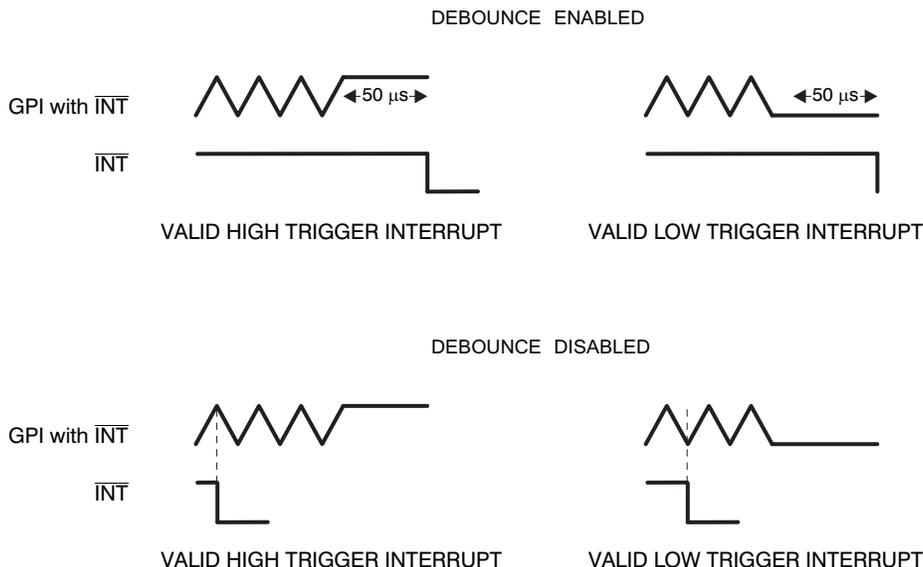
Debounce disable will have the same effect for GPI mode or for rows in keypad scanning mode. The  $\overline{\text{RESET}}$  input always has a 50-µs debounce time.
