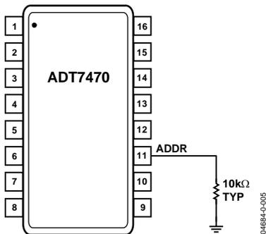
Figure 5. SMBus Address = 0x58 or 0x2C (Pin 11 = 0)
