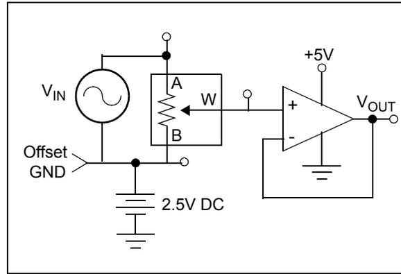
**FIGURE 2-64:** -3 db Gain vs. Frequency Test.
