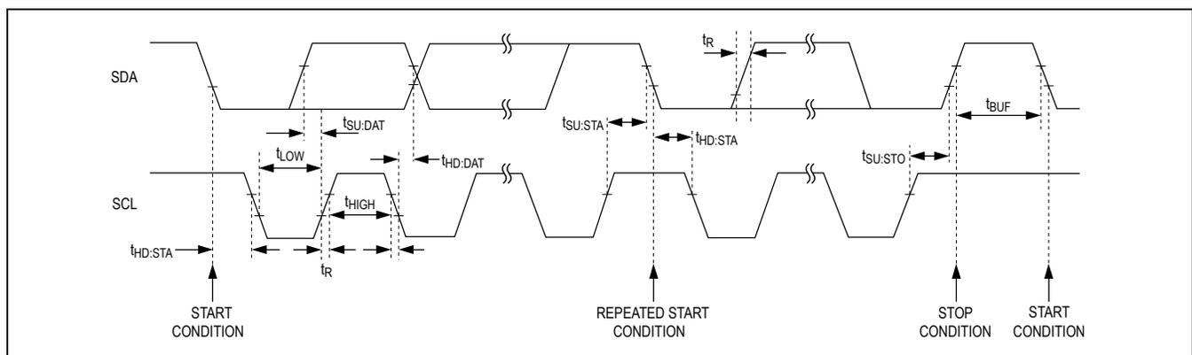
Figure 4. I<sup>2</sup>C Interface Timing Details
