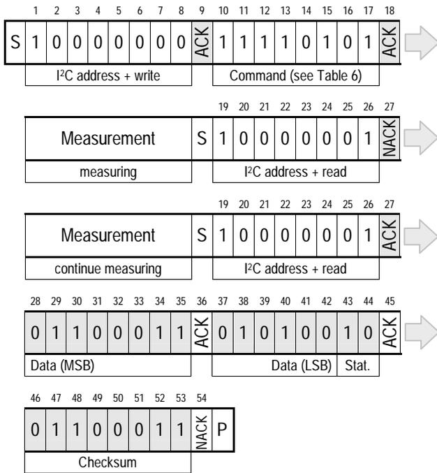
**Figure 14** No Hold master communication sequence – grey blocks are controlled by SHT2x. If measurement is not completed upon “read” command, sensor does not provide ACK on bit 27 (more of these iterations are possible). If bit 45 is changed to NACK followed by Stop condition (P) checksum transmission is omitted.
