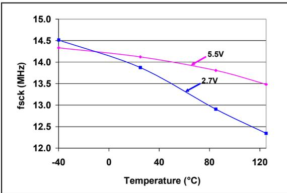
**FIGURE 2-63:** SCK Input Frequency vs. Voltage and Temperature.
