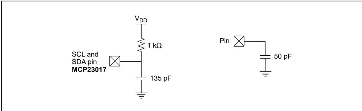
**FIGURE 1-1:** Load Conditions for device Timing Specifications.
