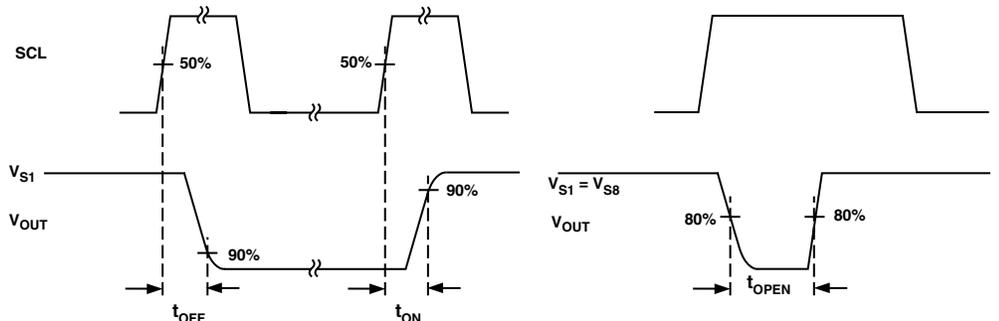
Test Circuit 5. Switching Times and Break-Before-Make Times
