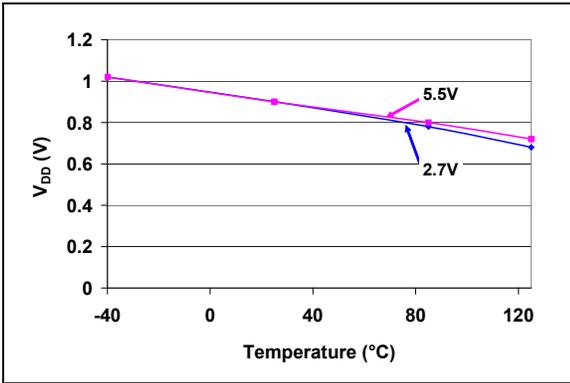
**FIGURE 2-62:** POR/BOR Trip point vs.  $V_{DD}$  and Temperature.
