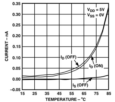
Figure 7. Leakage Currents as a Function of Temperature
