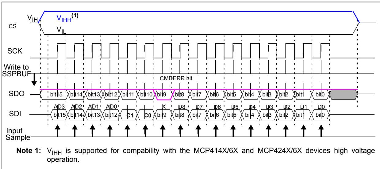
**FIGURE 6-4:** 16-Bit Commands (Write, Read) - SPI Waveform (Mode 0,0).
