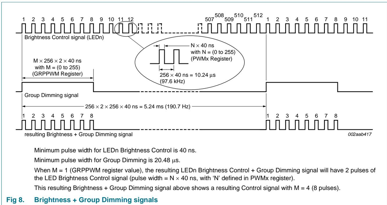
Fig 8. Brightness + Group Dimming signals
