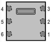
**Table 2** SHT2x pin assignment, NC remain floating (top view)
