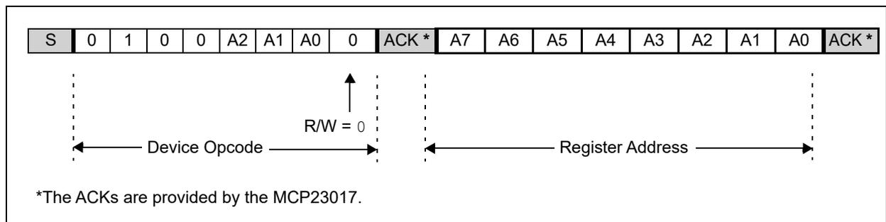
FIGURE 3-6: I<sup>2</sup>C Addressing Registers.
