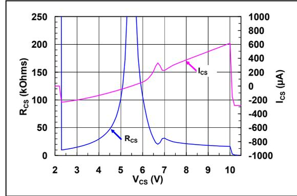
**FIGURE 2-3:**  $\overline{\text{CS}}$  Pull-up/Pull-down Resistance ( $R_{\overline{\text{CS}}}$ ) and Current ( $I_{\overline{\text{CS}}}$ ) vs.  $\overline{\text{CS}}$  Input Voltage ( $V_{\overline{\text{CS}}}$ ) ( $V_{DD} = 5.5\text{V}$ ).
