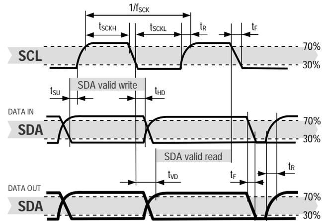
**Figure 10** Timing Diagram for Digital Input/Output Pads, abbreviations are explained in Table 5. SDA directions are seen from the sensor. Bold SDA line is controlled by the sensor, plain SDA line is controlled by the micro-controller. Both valid times (SDA read and SDA write) refer to the left SCL toggle.
