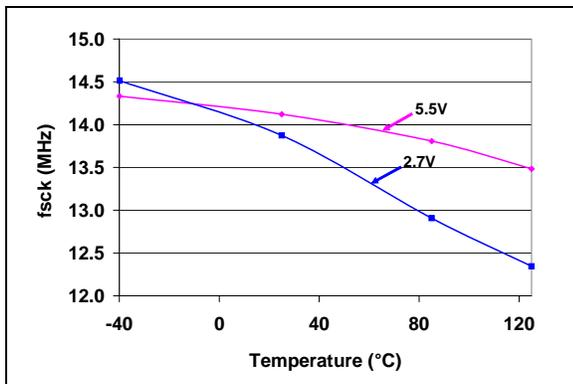
**FIGURE 2-57:** SCK Input Frequency vs. Voltage and Temperature.
