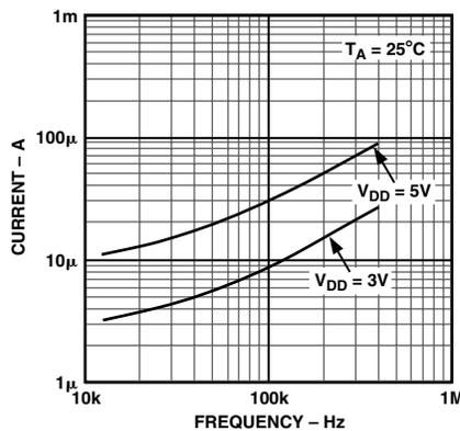
Figure 9. Input Current vs. Switching Frequency
