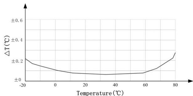
Figure 3: The maximum temperature error of temperature sensor
