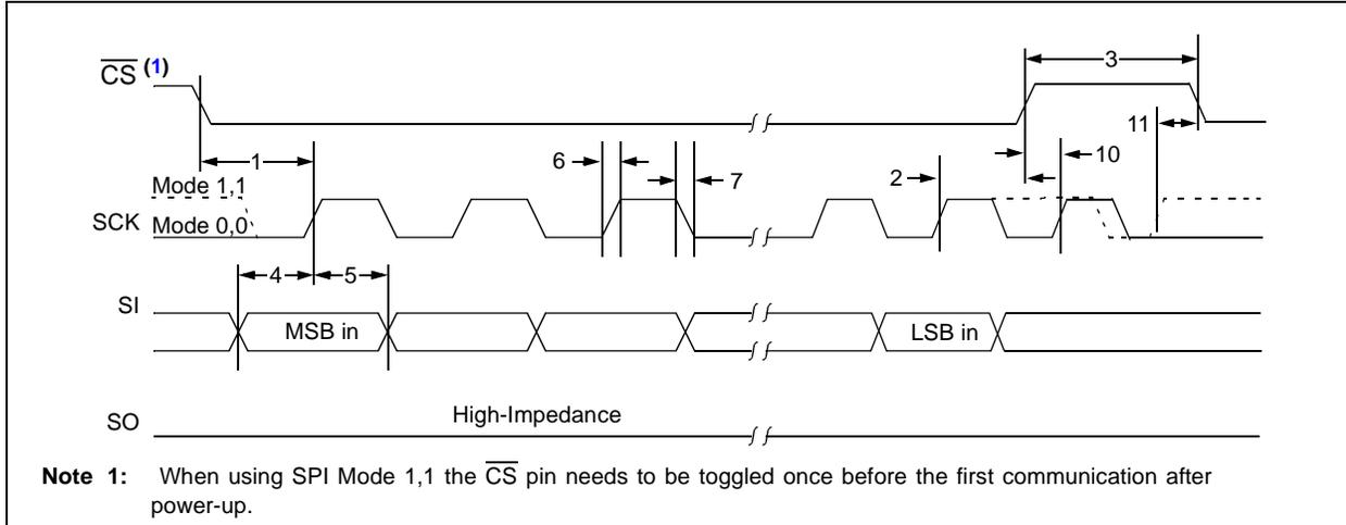
**FIGURE 1-6: SPI OUTPUT TIMING**
