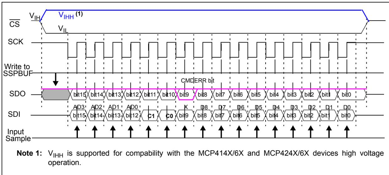
**FIGURE 6-3:** 16-Bit Commands (Write, Read) - SPI Waveform (Mode 1,1).
