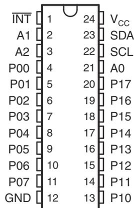
**Figure 5-1. DB, PW (TSSOP) Package
