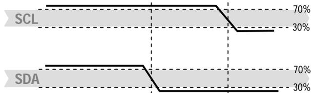
**Figure 11** Transmission Start Condition (S) - a high to low transition on the SDA line while SCL is high. The Start condition is a unique state on the bus created by the master, indicating to the slaves the beginning of a transmission sequence (bus is considered busy after a Start).
