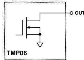
Figure 29. TMP06 Digital Output Structure
