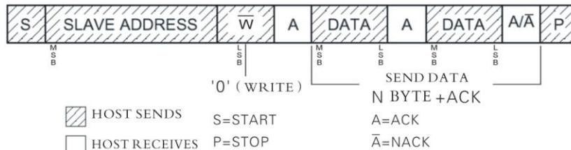
Figure 10: I<sup>2</sup>C The bus master sends data to the basic format from
