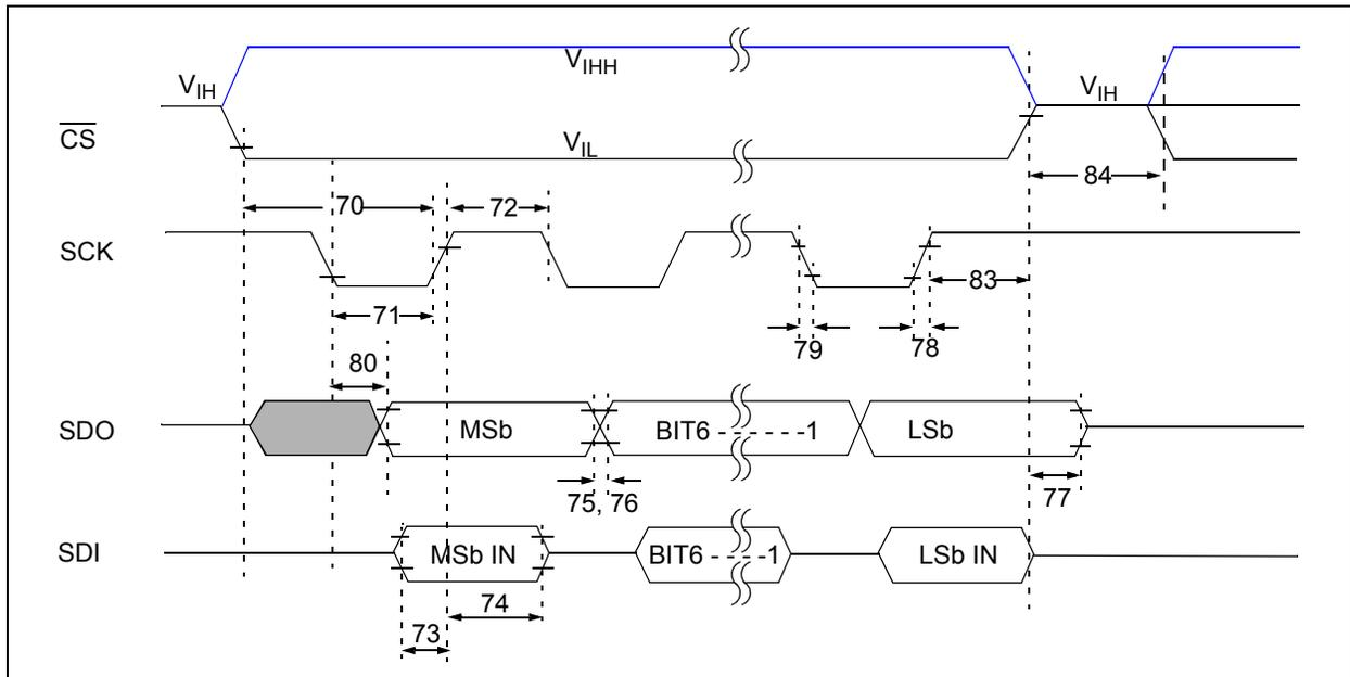
**FIGURE 1-1:** SPI Timing Waveform (Mode = 11).
