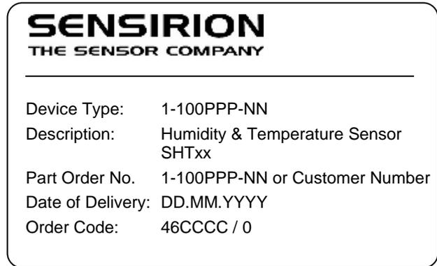
**Figure 21:** Second label on reel: For Device Type and Part Order Number (See Packaging Information on page 2), Delivery Date (also Date Code) is date of packaging of sensors (DD = day, MM = month, YYYY = year), CCCC = Sensirion order number.
