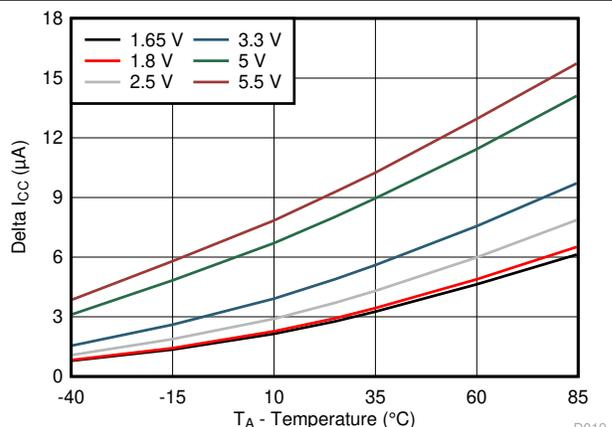
Figure 6-18. Δ I<sub>CC</sub> vs Temperature for Different V<sub>CC</sub> (V<sub>I</sub> = V<sub>CC</sub> – 0.6 V)
