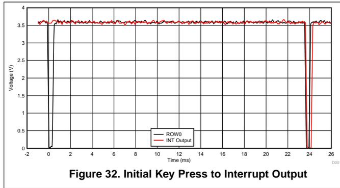
Figure 32. Initial Key Press to Interrupt Output
