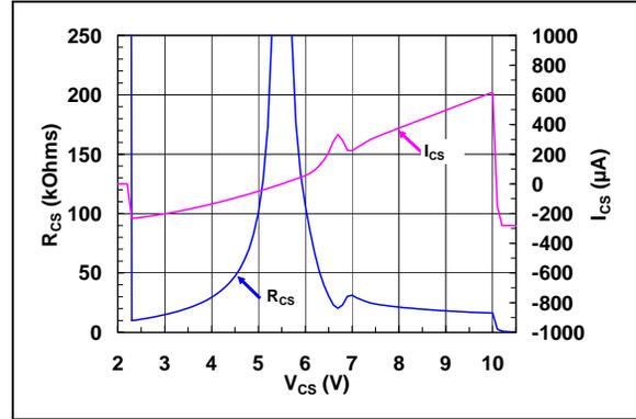
**FIGURE 2-4:**  $\overline{CS}$  Pull-up/Pull-down Resistance ( $R_{\overline{CS}}$ ) and Current ( $I_{\overline{CS}}$ ) vs.  $\overline{CS}$  Input Voltage ( $V_{\overline{CS}}$ ) ( $V_{DD} = 5.5\text{V}$ ).
