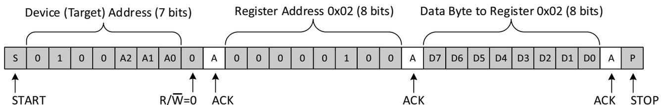
Figure 7-6. Write to the Polarity Inversion Register
