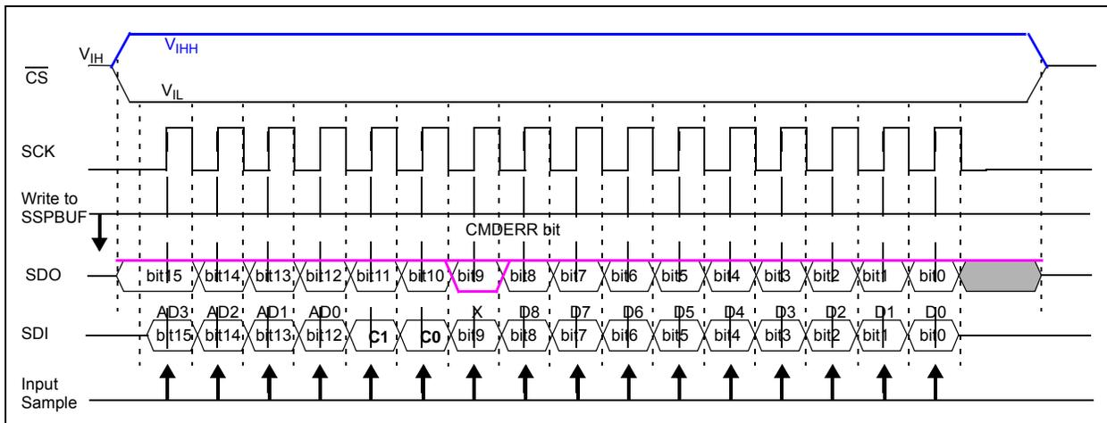
FIGURE 6-4: 16-Bit Commands (Write, Read) - SPI Waveform (Mode 0,0).
