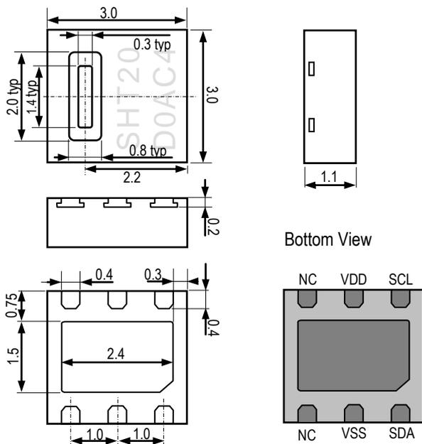
**Figure 1:** Drawing of SHT20 sensor package, dimensions are given in mm (1mm = 0.039inch), tolerances are  $\pm 0.1$ mm. The die pad (center pad) is internally connected to VSS. The NC pads must be left floating. VSS = GND, SDA = DATA. Numbering of E/O pads starting at lower right corner (indicated by notch in die pad) and goes clockwise (compare Table 2).
