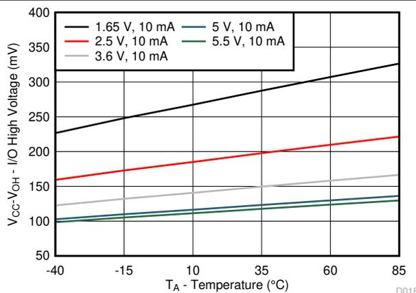
Figure 6-17. V<sub>CC</sub> – V<sub>OH</sub> Voltage vs Temperature for Different V<sub>CC</sub>
