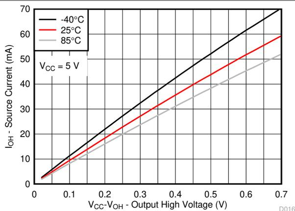
Figure 6-15. I/O Source Current vs Output High Voltage for Different Temperature (T<sub>A</sub>) for V<sub>CC</sub> = 5 V
