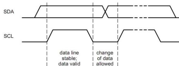
Figure 5: I<sup>2</sup>C Bus bit transmission
