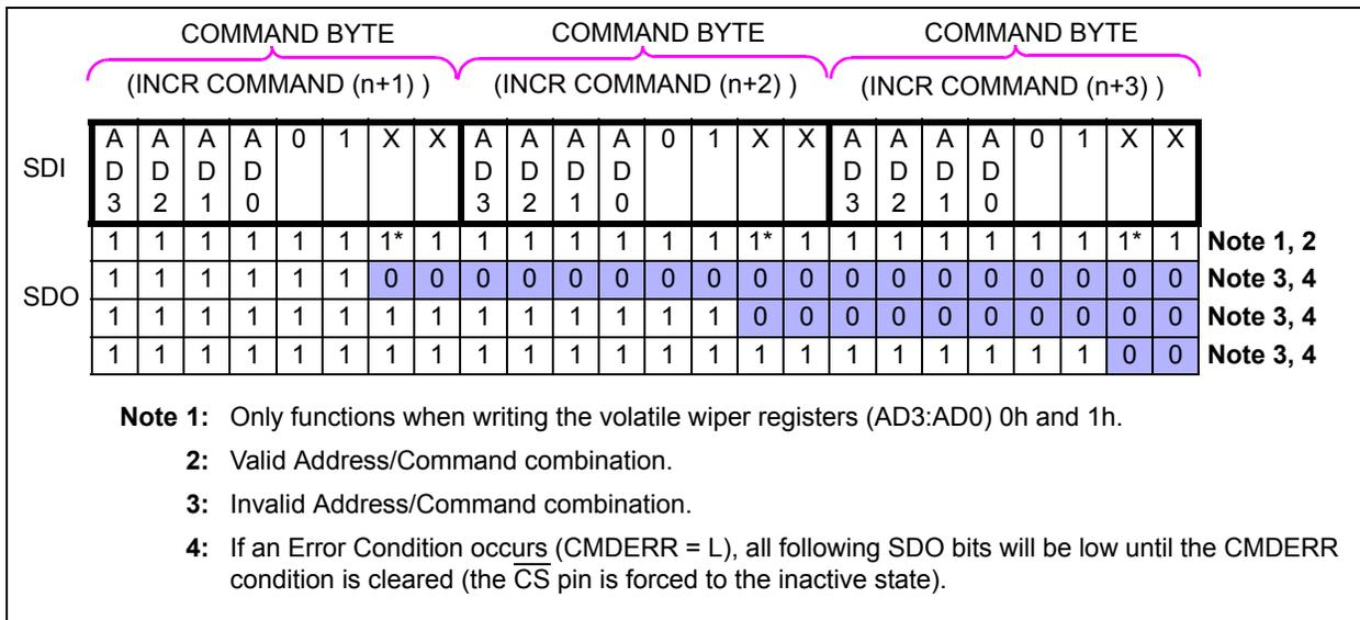
FIGURE 7-7: Continuous Increment Command - SDI and SDO States.
