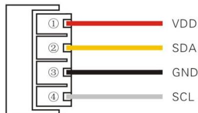
Figure 1: AM2315wiring diagram
