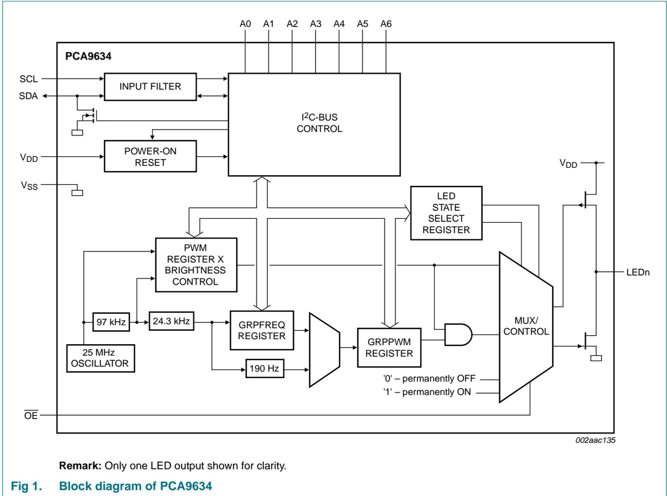
Fig 1. Block diagram of PCA9634
