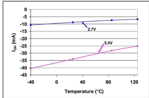
**FIGURE 2-53:**  $I_{OH}$  (SDO) vs.  $V_{DD}$  and Temperature.
