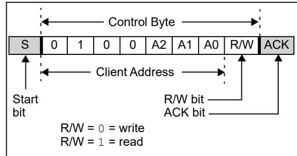
FIGURE 3-4: I<sup>2</sup>C Control Byte Format.
