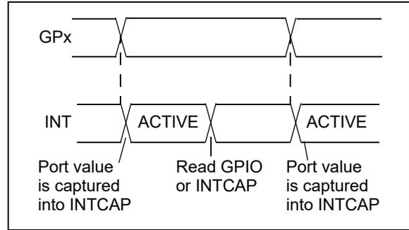
**FIGURE 3-8:** Interrupt-on-Pin Change.
