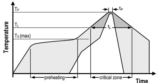
**Figure 9** Soldering profile according to JEDEC standard.  $T_P \leq 260^\circ\text{C}$  and  $t_P < 30\text{sec}$  for Pb-free assembly.  $T_L < 220^\circ\text{C}$  and  $t_L < 150\text{sec}$ . Ramp-up/down speeds shall be  $< 5^\circ\text{C}/\text{sec}$ .
