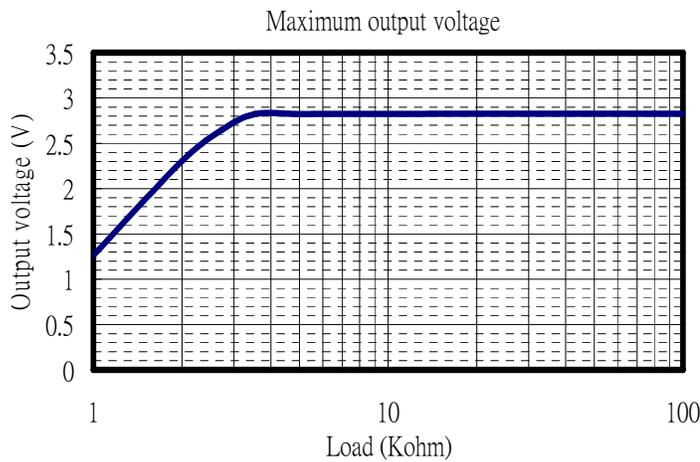
Maximum Output Level VS R<sub>LOAD</sub>
