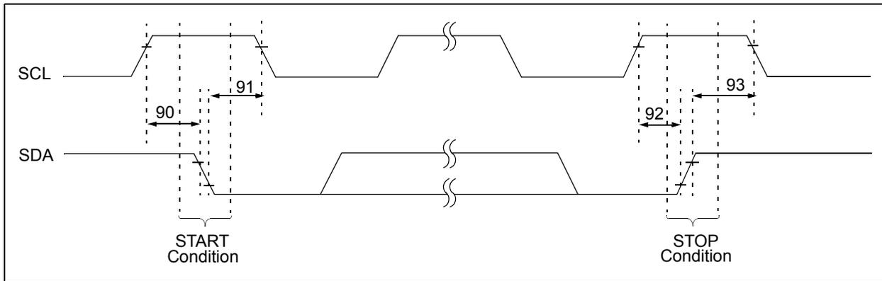
**FIGURE 2-4: I<sup>2</sup>C™ BUS DATA TIMING**
