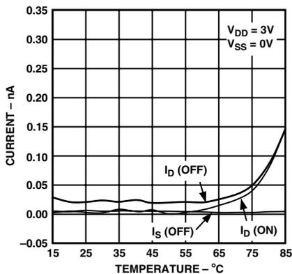
Figure 8. Leakage Currents as a Function of Temperature
