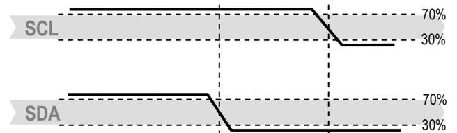
**Figure 13** Transmission Start condition (S) - a high to low transition on the SDA line while SCL is high. The Start condition is a unique state on the bus created by the master, indicating to the slaves the beginning of a transmission sequence (bus is considered busy after a Start).
