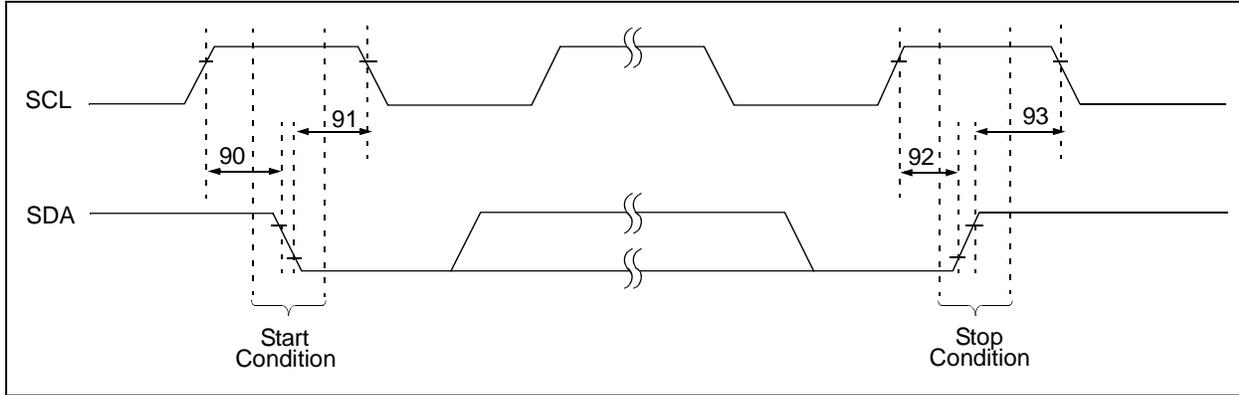
**FIGURE 1-4: I<sup>2</sup>C BUS DATA TIMING**
