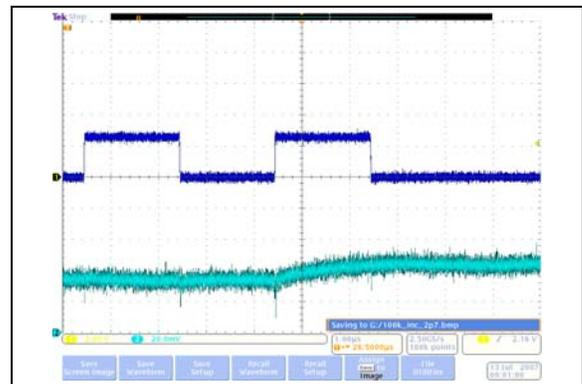
**FIGURE 2-53:** 100 k $\Omega$  – Power-Up Wiper Response Time (1  $\mu\text{s}/\text{Div}$ ).
