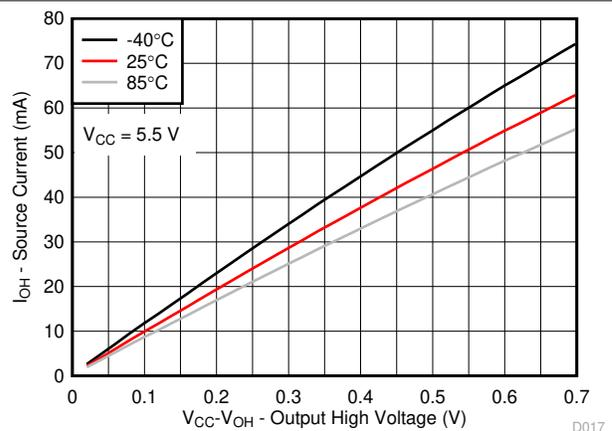
Figure 6-16. I/O Source Current vs Output High Voltage for Different Temperature (T<sub>A</sub>) for V<sub>CC</sub> = 5.5 V
