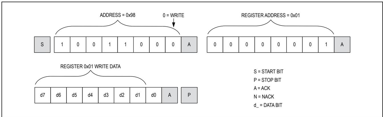
Figure 8. Format for I<sup>2</sup>C Write
