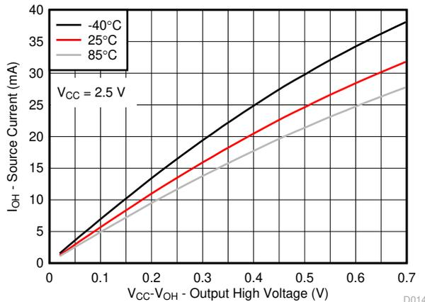
Figure 6-13. I/O Source Current vs Output High Voltage for Different Temperature (T<sub>A</sub>) for V<sub>CC</sub> = 2.5 V
