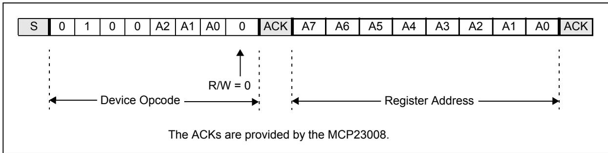
**FIGURE 1-5: SPI ADDRESSING REGISTERS**
