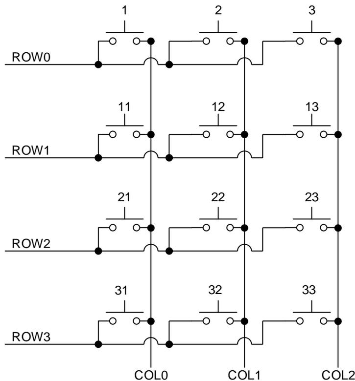
**Figure 31. Keypad Schematic**
