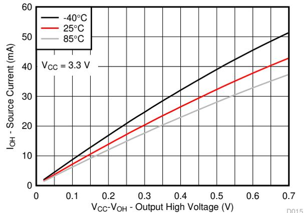
Figure 6-14. I/O Source Current vs Output High Voltage for Different Temperature (T<sub>A</sub>) for V<sub>CC</sub> = 3.3 V
