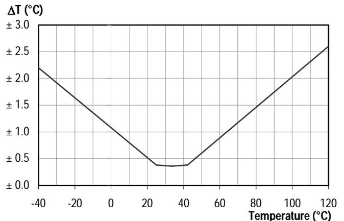
**Figure 3** Maximal tolerance for temperature sensor in °C.
