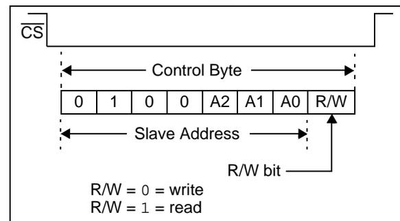
**FIGURE 3-6: I<sup>2</sup>C ADDRESSING REGISTERS**
