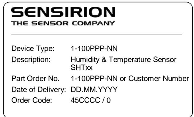
**Figure 19:** Second label on reel: For Device Type and Part Order Number (See Packaging Information on page 2), Delivery Date (also Date Code) is date of packaging of sensors (DD = day, MM = month, YYYY = year), CCCC = Sensirion order number.
