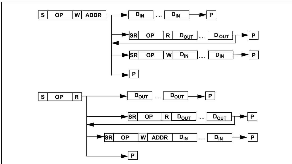
FIGURE 3-3: MCP23017 I<sup>2</sup>C Device Protocol.
