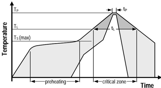
**Figure 7** Soldering profile according to JEDEC standard.  $T_p \leq 260^\circ\text{C}$  and  $t_p < 40\text{sec}$  for Pb-free assembly.  $T_L < 220^\circ\text{C}$  and  $t_L < 150\text{sec}$ . Ramp-up/down speeds shall be  $< 5^\circ\text{C}/\text{sec}$ .
