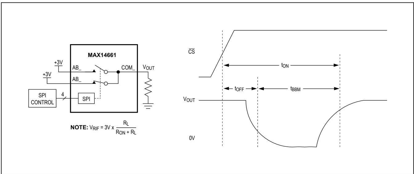
Figure 2. Turn-On/Turn-Off/Break-Before-Make
