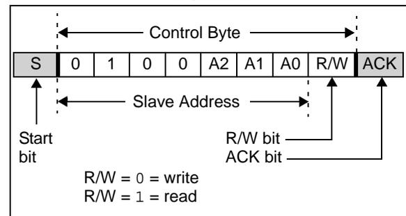
**FIGURE 3-5: SPI CONTROL BYTE FORMAT**
